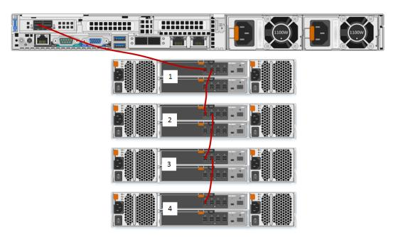
5. When you finish the cabling, ensure that the PowerVault is powered on and then power on the host.
