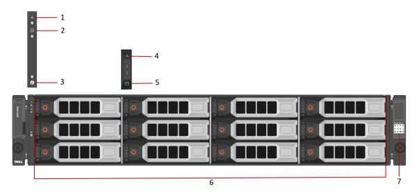
Item numbers 1-3 are indicators located on the front control panel, which indicate the status of the enclosure. Item numbers 4-5 are hard disk drive indicators. For more detailed information, see The *Dell Storage MD1400 Enclosures Hardware Owner's Manual* (https://topics-cdn.dell.com/pdf/md1400om\_en-us.pdf).
