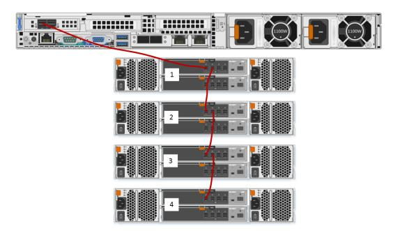
5. When you finish the cabling, ensure that the PowerVault is powered on and then power on the host.
