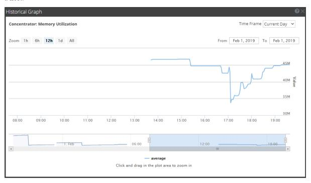
The graphical view is customized to display the statistics collected for the current day and the values are zoomed in for an interval of an hour (10.15 - 11.15 hrs). Hover over the graph to view the details at a particular instant. For example, in the figure it displays the memory utilization at 12.00 hrs.
