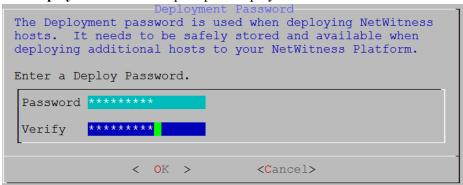
Type the Password, down arrow to Verify, retype the password, tab to OK, and press Enter.
