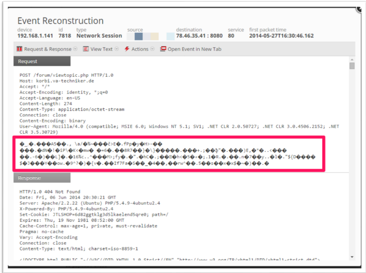
Figure 13. HTTP with Binary Data in Payload
