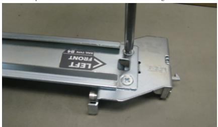
4. Remove the bracket and replace it with the new bracket.
