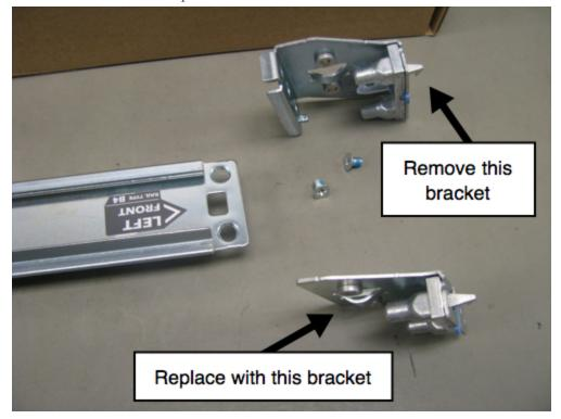
5. Re-use the screws to fasten the new bracket in place.
