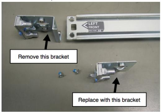
5. Re-use the screws to fasten the new bracket in place.
