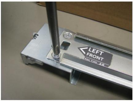
4. Remove the bracket and replace it with the new bracket.
