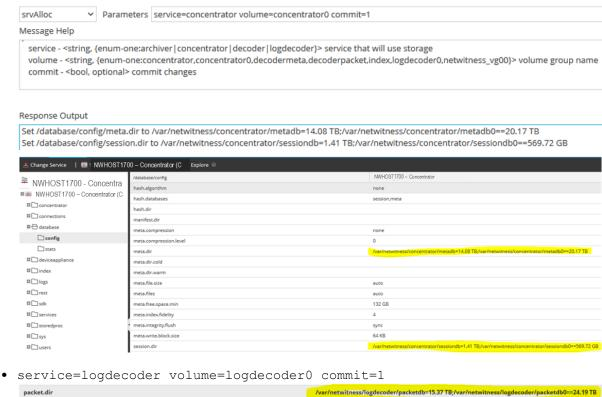
Reconfigure the following Log Decoder service and its database to detect and take advantage of all
