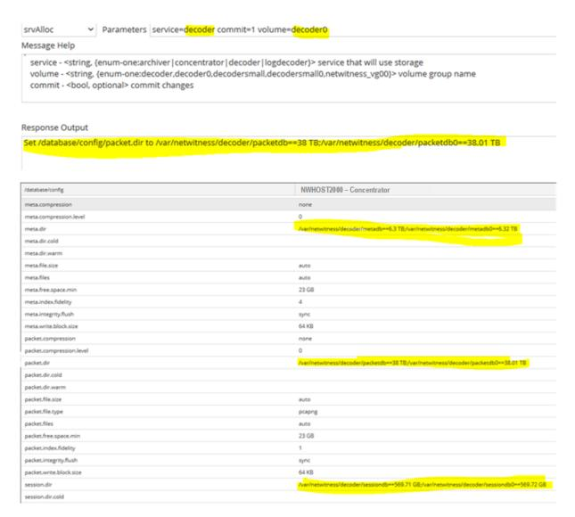
10. Reconfigure the following Network Decoder service and its database to detect and take advantage of all of the free space as described in <u>Task 5 - (Optional) Reconfigure Storage Configuration for 10G Capture</u>.
