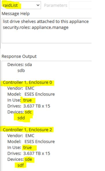
3. Use the raidList command to display block devices for enclosures so you can verify In Use: TRUE.
