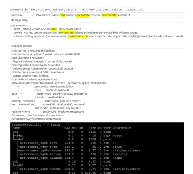
4. Execute the partNew command with the following parameters with the following parameters to create an index on SSDs.
