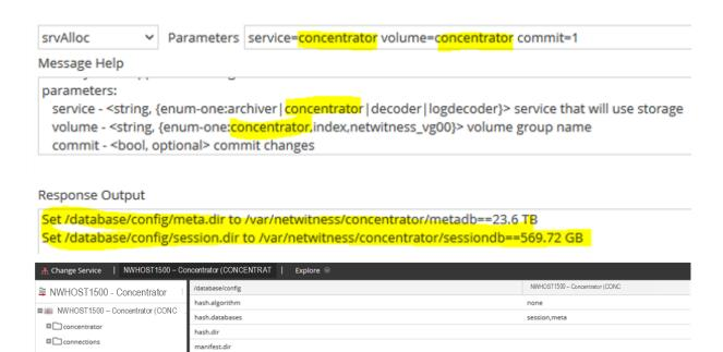
Reconfigure the following Network Concentrator service and its database to detect and take advantage of all of the free space as described in <a href="Task 5 - (Optional) Reconfigure Storage">Task 5 - (Optional) Reconfigure Storage</a> Configuration for 10G Capture.
